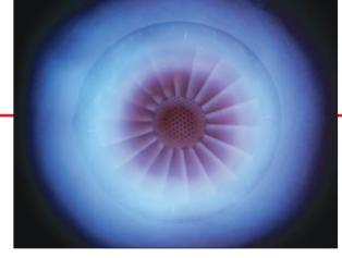
Unique firing head produces stable combustion and ultra low NOx when firing natural gas.
