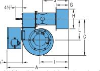
Add 3/8" to "H" for opening in heat exchanger front plate.
