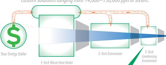
E-Tech condensing economizers yield extremely high efficiencies — upward of 96%. Their vapor-condensing environment presents an ideal heat recovery solution for industries that use non-sulfur bearing fuels, whose acidic byproducts can corrode most carbon and alloy materials. The cost-efficient way to convert water vapor to recaptured heat.
