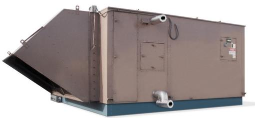
L.J. Wing SAS Steadyair® air handlers are reliable heating and ventilating make-up air packages. They provide all the advantages of the proven L.J. Wing IFB integral face and bypass coil, including positive freeze protection, accurate temperature control, constant air volume and elimination of stratification. These units also feature:
