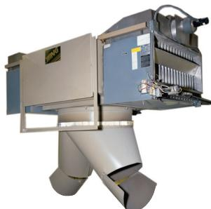
L.J. Wing GA Gas Assemblies are indirect-fired gas unit heaters that bundle two or four duct furnaces with an axial flow propeller fan and one of Wing's unique fixed or revolving discharges to provide a dependable source of heated air for large open space or door heating applications.
